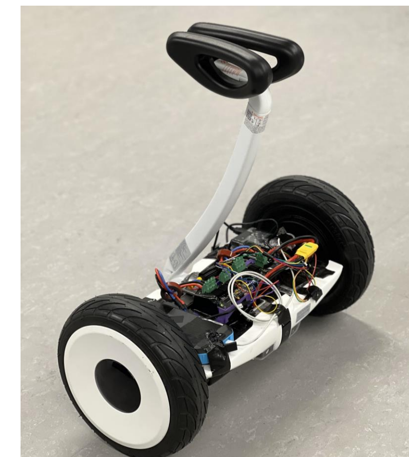
Figure 3: Modified Segway stabilizing autonomously
