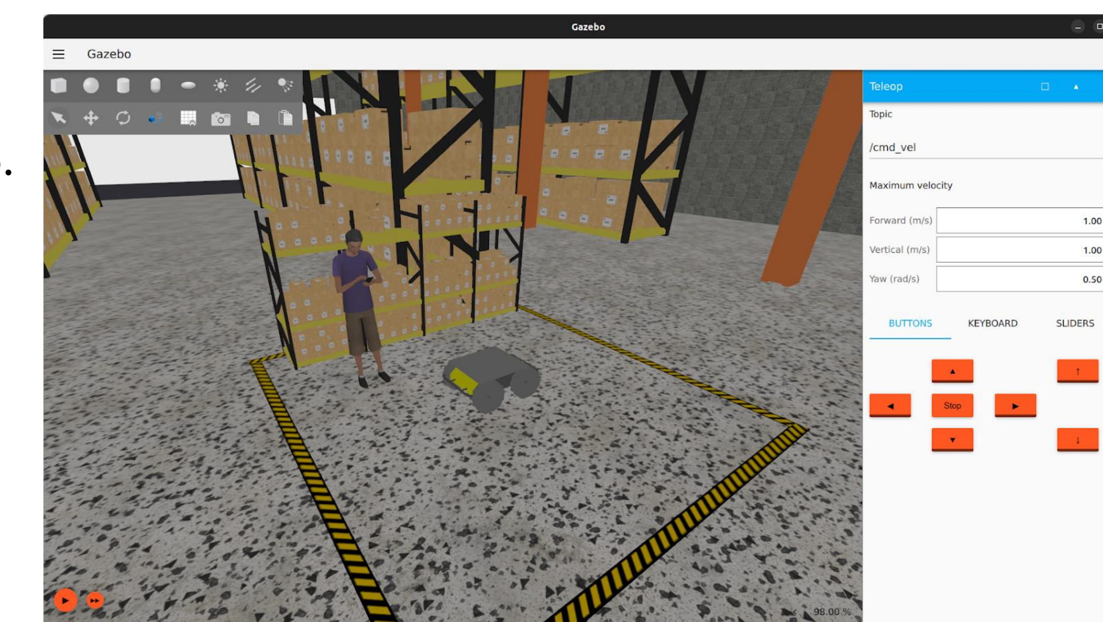
Figure 5: Screenshot of a Gazebo Simulation of the robot in a simulated environment
